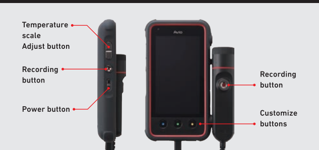
Frequent operation such as “Temperature Scale Setting” and “Recording” can be performed by hardware key. Comfortable one-hand measurement is possible even wearing gloves.
