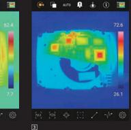
The setting and adjustment of temperature scale was the most difficult operation for beginners. With the new "Auto Point" function, even beginners can easily set the optimal temperature scale by touching the upper and lower limit temperature values intuitively. Moreover, you can automatically adjust the upper limit temperature values which depends on the temperature change by "Auto-Maximum" function.
